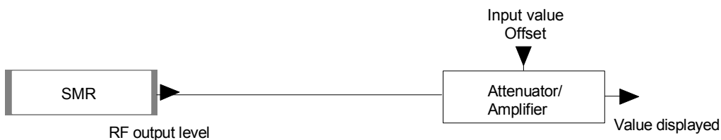
Fig. 4-4 Typical setup with level offset
